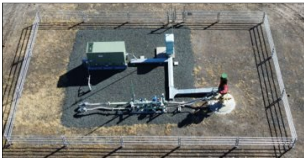
Figure 9 Typical well configuration
