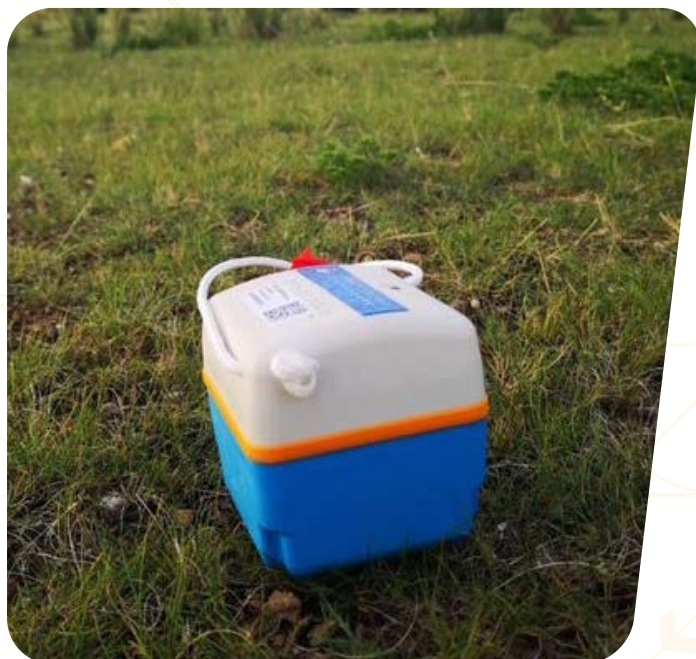
Small wireless geophones are spiked into the ground every 5-20m along the survey line.
