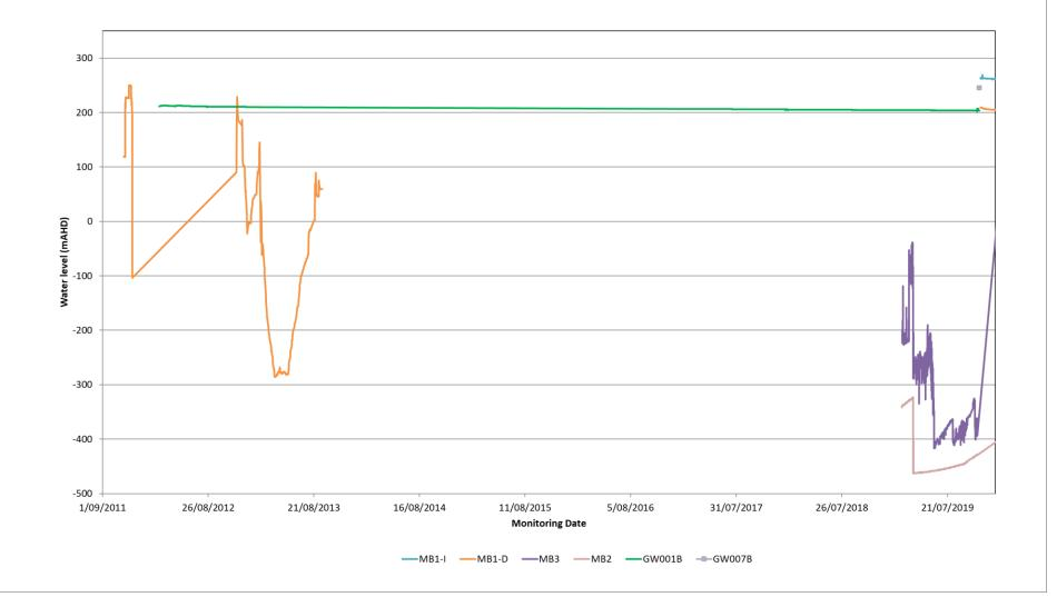
Figure 6: BGP Deep Bores Water Pressure Monitoring Results - 2012 to present
