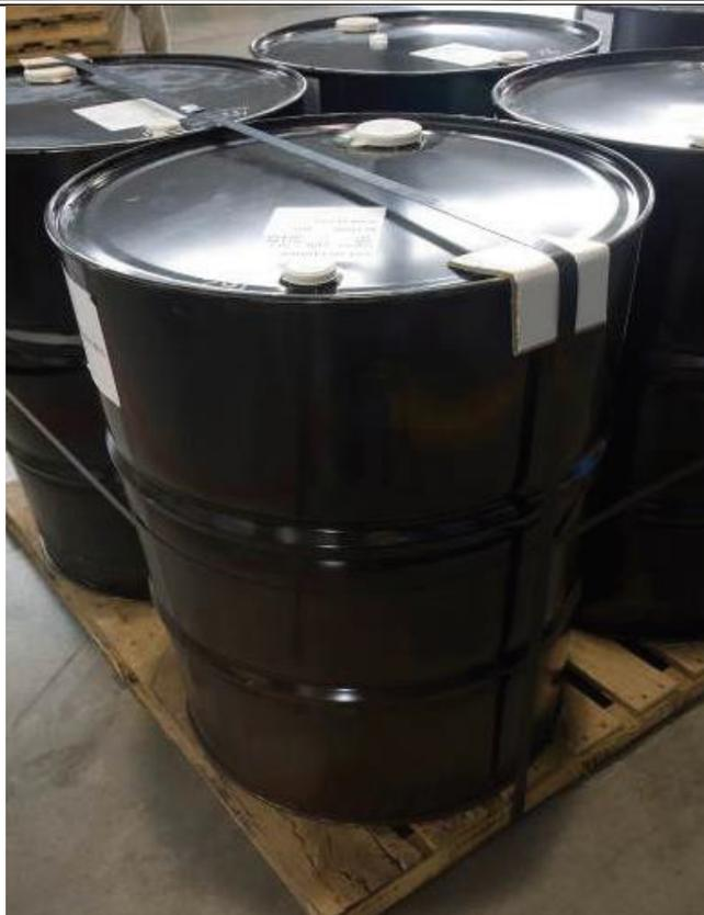
Drums properly secured to pallet under bearers
