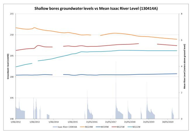
Figure 11: Shallow Groundwater levels vs mean Isaac River levels
