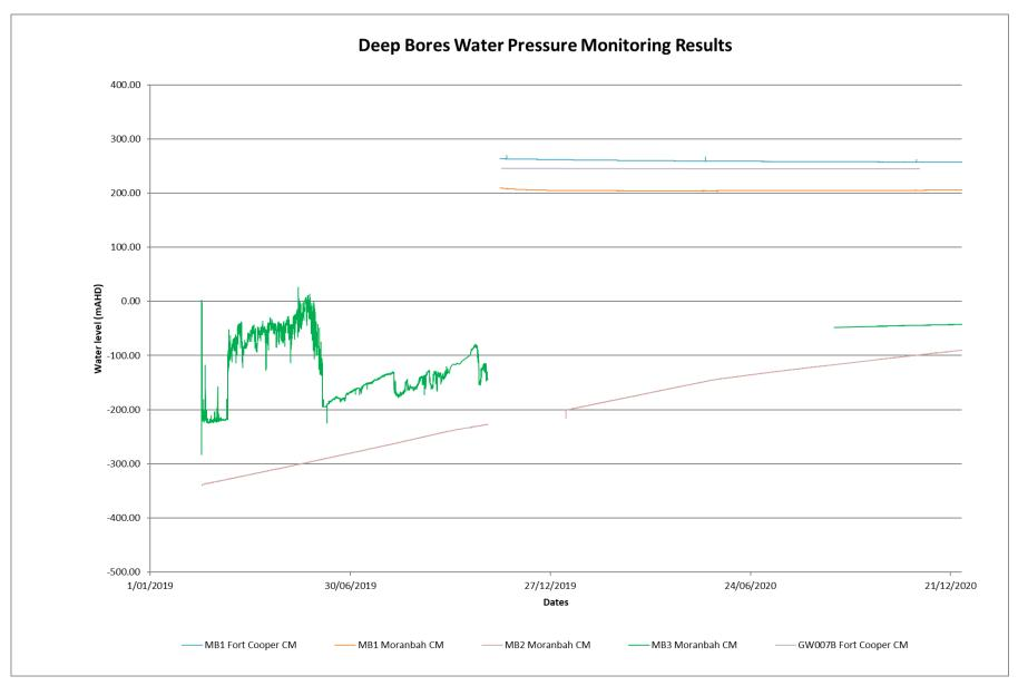
Figure 13: Deep Bores Water Level Monitoring Results - BGP
