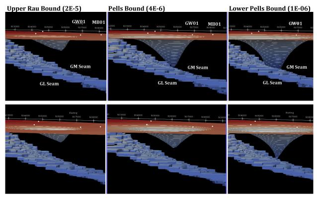
Figure 5.1 Cross section of GM head pressure (April 2024 and September 2027)
