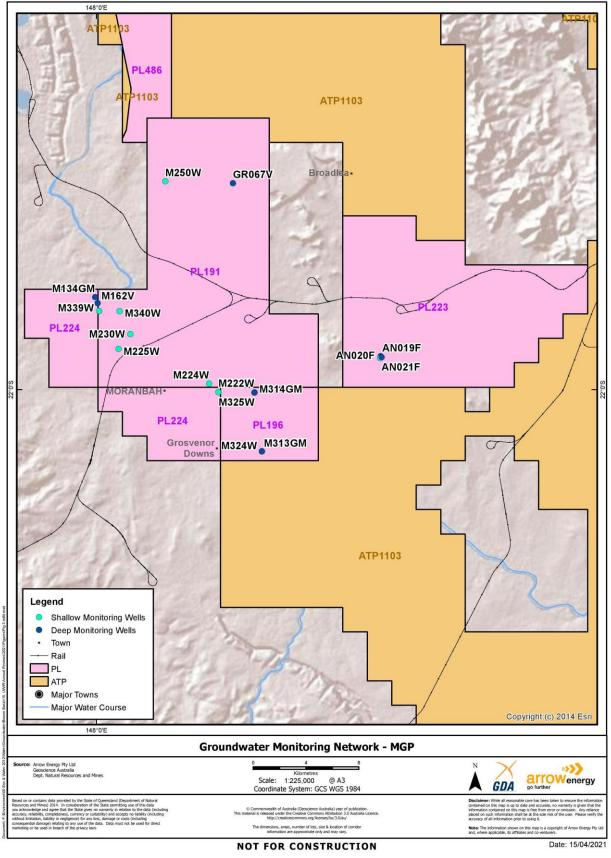
Figure 3: Groundwater Monitoring Network for MGP
