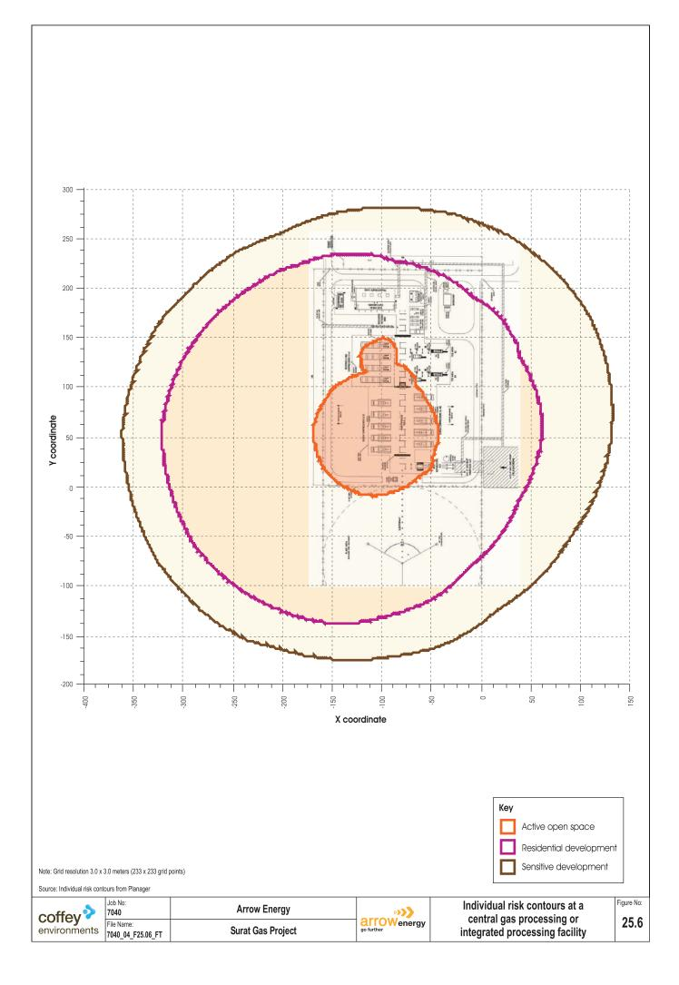
The risk of injury and propagation from a central gas and integrated processing facility extends up to 30 m from the outer edge of the compressors. Given a typical site layout, it is unlikely that this distance would extend beyond the site boundary as shown in Figure 25.7. The risk of injury and propagation for this type of facility is considered to be **low**.
