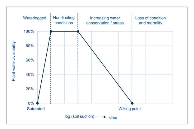
Figure 6-6 Soil water availability as a function of soil suction and its resultant ecological effects<sup>2</sup>
