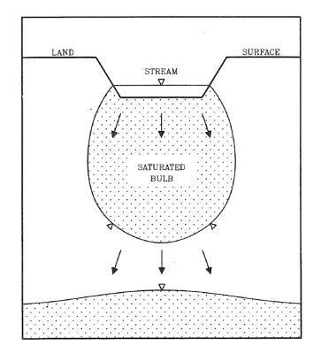
Figure 5-2 Disconnection below a stream without a clogging layer (from Peterson and Wilson 1988)
