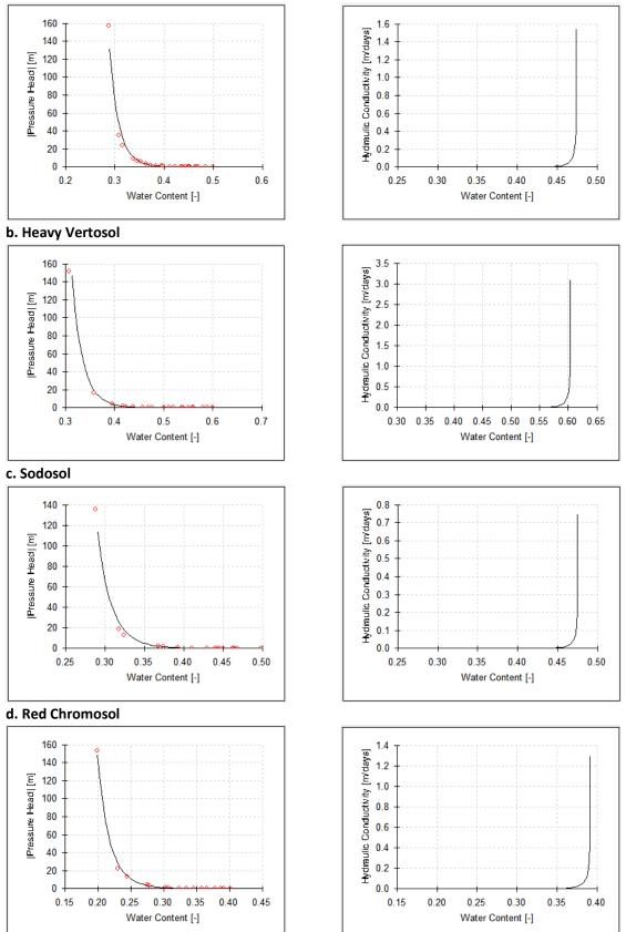
Figure B-2 Measured water retention data (red symbols) from Connolly et al. (1997) fitted to the van Genuchten-Mualem model using the RETC code
