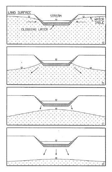
Figure 5-1 Stream-aquifer interaction with a clogging layer (a) connected gaining stream, (b) connected losing stream, (c) disconnected stream with a shallow water table, and (d) disconnected stream with a deep water table (from Peterson and Wilson 1988)
