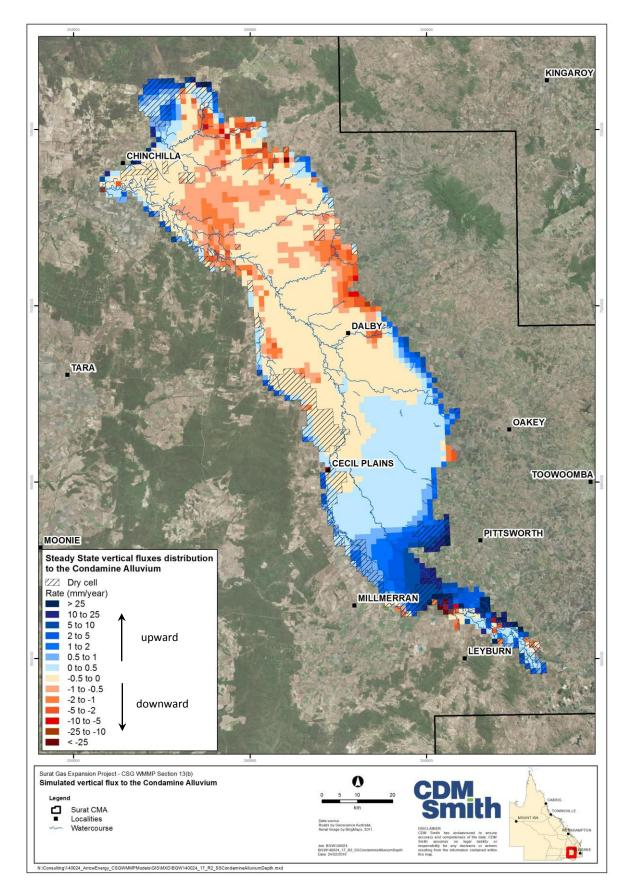
Figure 7-5 Surat CMA groundwater model, NSMC realisation r1 - simulated vertical flux to the Condamine Alluvium for the steady state initial condition
