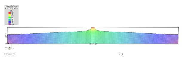
Figure B-3 Example FEFLOW result for saturated flow (free and movable water table) and anisotropy ratio 100
