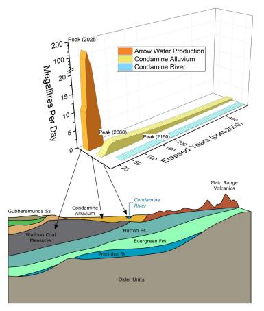
Predicted groundwater fluxes induced by Arrow for the high-case model realisation
