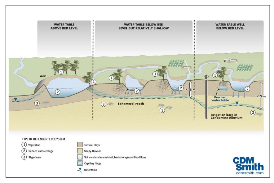
Figure 6-7 Different hydrological settings in the Condamine Alluvium relative to DE Types
