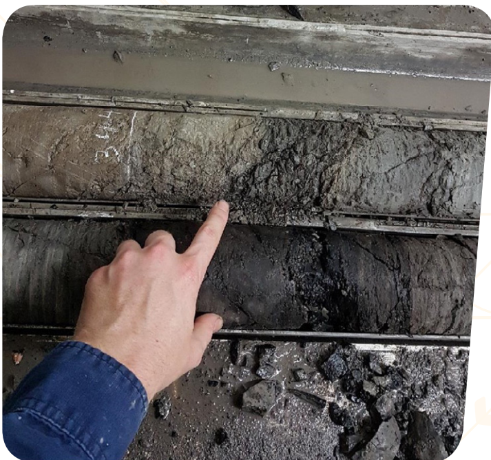
Plainview 34 core showing the fault zone and 'fault gouge'
