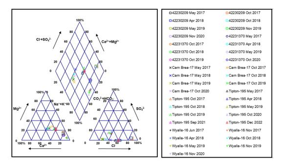
Figure 3-18: Condamine Alluvium Piper Diagram
