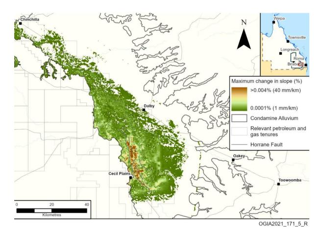
Figure 3-26: Predicted maximum change in ground slope from CSG-induced subsidence within the Condamine Alluvium area (after OGIA, 2021)
