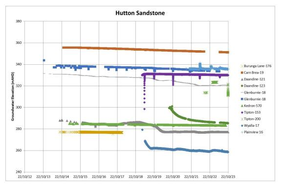
Figure 3-4: Hutton Sandstone monitoring bores hydrograph
