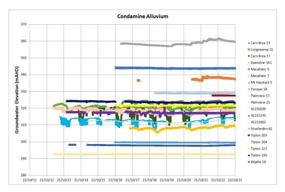
Figure 3-1: Condamine Alluvium monitoring bores hydrograph
