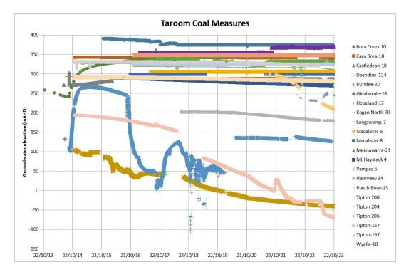
Figure 3-9: Taroom Coal Measures monitoring bores hydrograph
