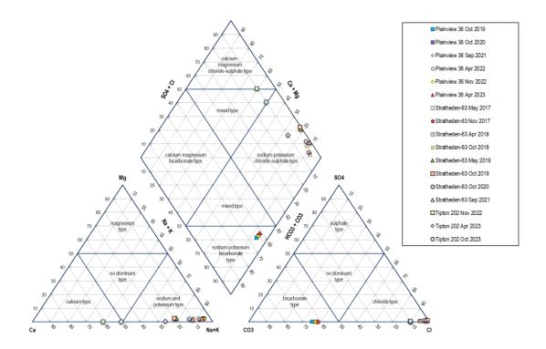
Figure 3-20: Springbok Sandstone Piper Diagram
