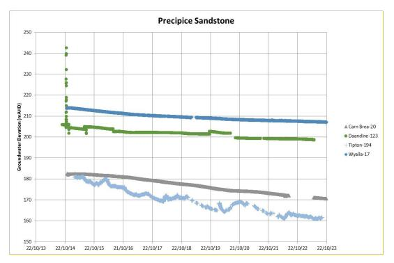
Figure 3-5: Precipice Sandstone monitoring bores hydrograph
