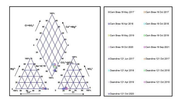
Figure 3-22: Hutton Sandstone Piper Diagram
