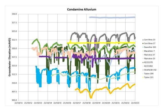
Figure 3-2: Central Condamine Alluvium area monitoring bores hydrograph
