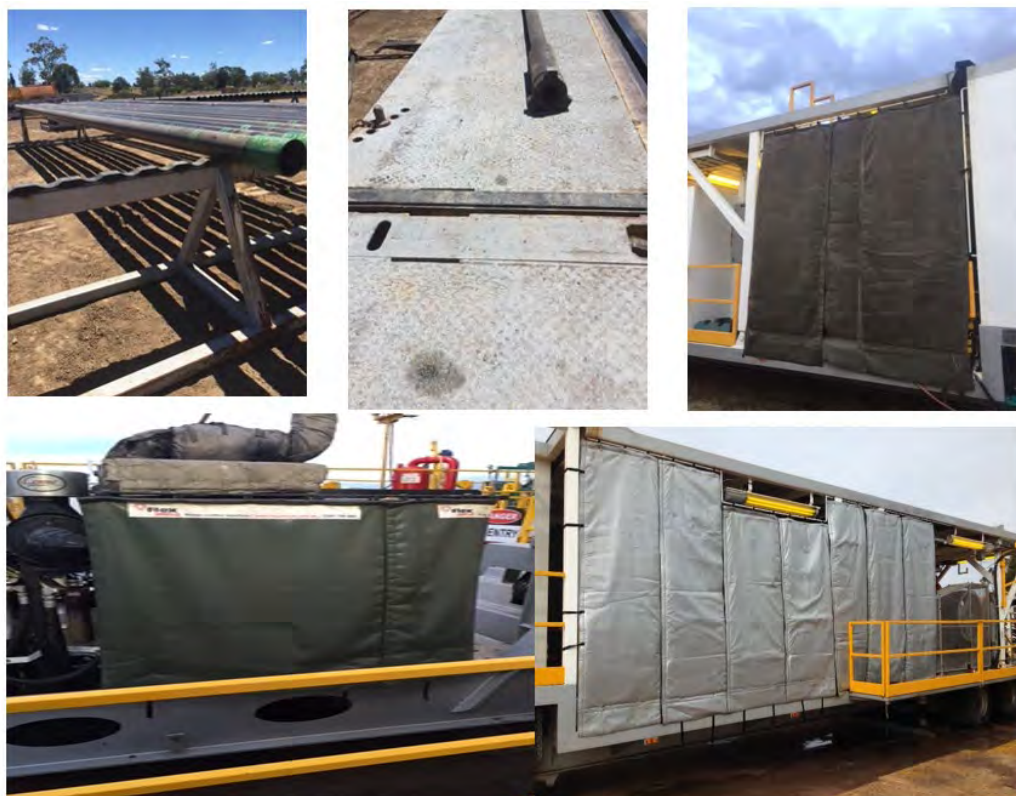
Figure 6: Examples of noise attenuation measures included in rig activities contracted to operate on Arrow Energy gas fields.
