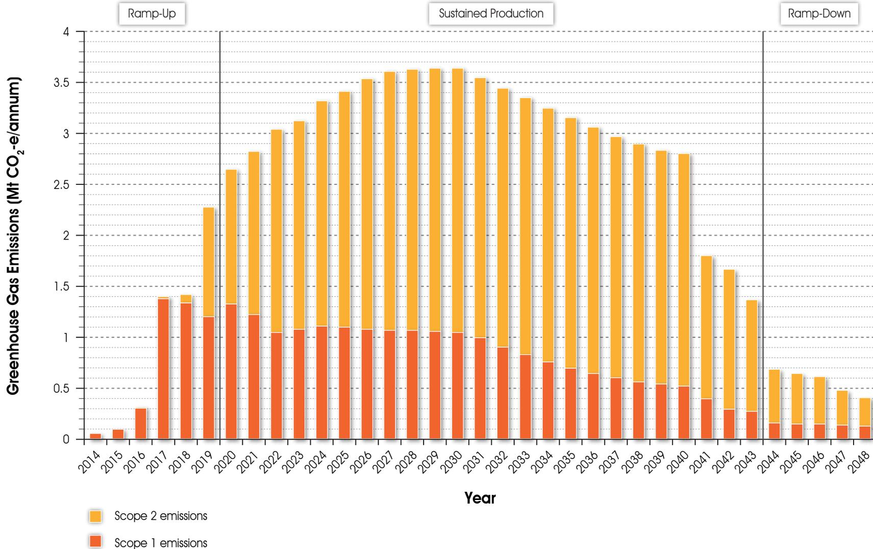
Scope 1 emissions are higher during ramp-up due to the combustion of fuel for power generation in the early stages of the project. A significant increase in Scope 2 emissions is then predicted when the production facilities and wells are connected to the Queensland electricity grid for the sustained production and ramp-down phases of the project.
